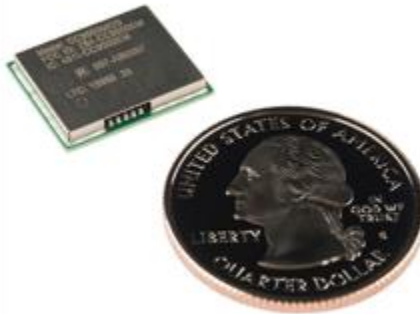
Figure 4.2.1-4: Wi-Fi Module (used with permission from SparkFun Electronics)
